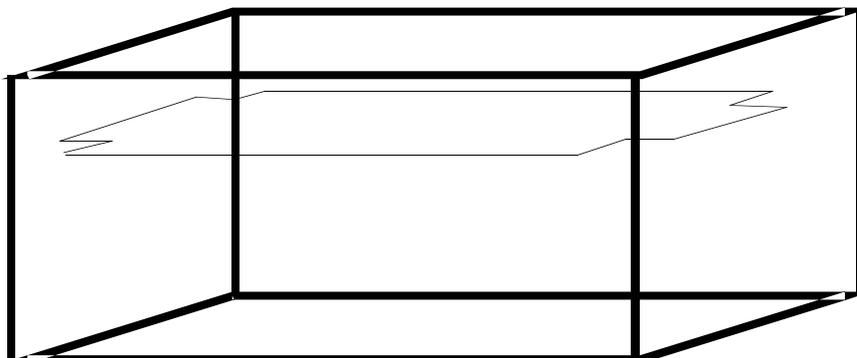
If there is a steel-reinforcing grid in the floor, either put the loop in the ceiling or, if it must go in the floor, install the loop in plastic conduit as far above the grid as possible. The drive current may have to be turned up to overcome the effects of the metal, so choose the largest conductor size possible to suit the area.
