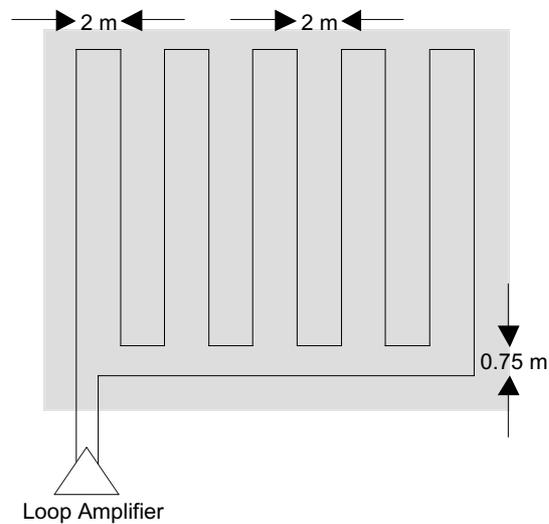
The gap between the prongs of the pattern is about 2 metres because this reduces the overspill (left - right in the diagram) to about six metres but allows the field to spread upwards enough to give good coverage at head height. The up - down overspill as shown in the diagram will be slightly more than the left — right spill but will still be a lot less than for a simple rectangular pattern.
