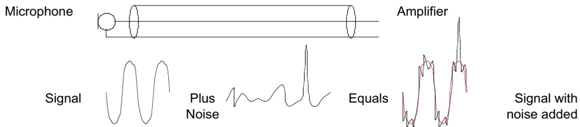
The microphone cable, despite being screened, acts as an aerial and picks up electrical noise very easily. This noise can be a low hum, such as from the electrical mains, or loud cracks, such as those caused by sparking light switches.
