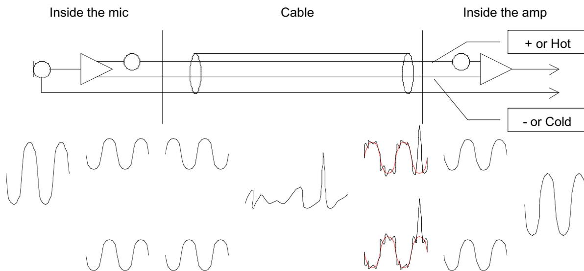
Signal from mic. Split signal. Invert one line, pass down balanced line, interference on both lines.
