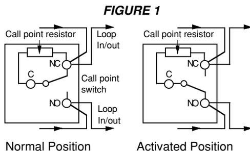
**Note:** Resistors are not included with the panel but are available from electronic component suppliers. Failure to include this resistor will cause the panel to show a short circuit fault indication when the call point is operated. This also applies to any other form of switch used to trigger the detector circuits. This panel will work with resistance values from 470 to 680 ohms fitted. The resistors must be rated half watt.
