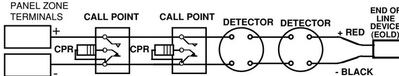
**\*THREE WIRE SYSTEM** Combined detector and sounder loops using common 0v conductor.
