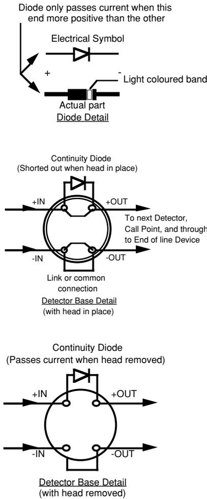
The diode must be connected so that it is shorted out by the internal connections of the head when the head is in place, and provides a path for the current in the loop when the head is removed. Incorrect fitting will not cause damage but will cause malfunctions of the system. (See troubleshooting - page 9)
