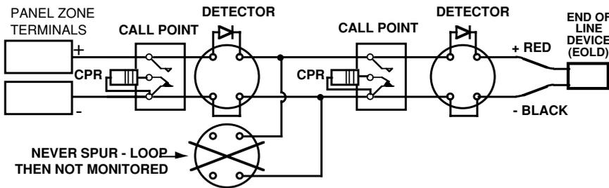
**ZONE LOOP CIRCUIT** (Call points wired before detectors) detector base diodes not needed -
